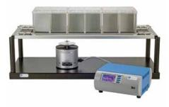
The Plantar Test Instrument (Hargreave's Method) measures response to infrared heat stimulus, applied to the plantar surface. Our Plantar Test is the original apparatus, designed in close cooperation with Prof. Ken Hargreaves, who devised the method. Latency to paw withdrawal and infrared intensity are recorded automatically (i.e.no manual scoring, as in other models available on the market!).
