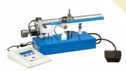
The Ugo Basile original design of this classic device dates back to the 1960s. The Analgesy-Meter performs Paw Pressure experiments according to the Randall-Selitto method for a rapid and sensitive screening of analgesic and anti-inflammatory drug. The force is applied to the animal paw, by a cone-shaped pusher with a rounded tip, which does not hurt the animal. The 37215, originally designed for rats, is conveniently used also with mice.
