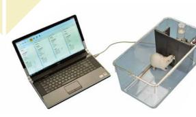
The **Orofacial Stimulation Test** by Ugo Basile is a new method to measures hypersensitivity to thermal or mechanical stimulation of the trigeminal area in rats; animals are trained & tested in standard home cages.
